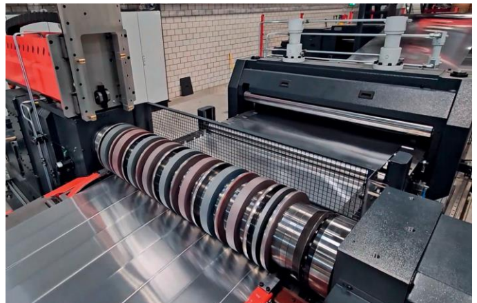
Strips are slit with minimal burr formation
