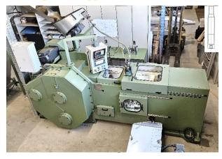
The press is designed for heading and indenting steel or brass ammunition cases. Any other forward or backward extrusion operations can be produced on this machine.
