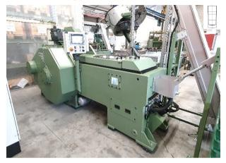
This press is designed for the drawing of ammunition cases made of steel or brass.
